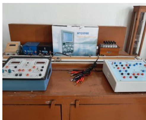
Set ups for 1) (Back) determining unknown resistance using meter bridge, 2) (L) setup to study characteristics of P-N junction diode, 3) (R) OPAMP setup for integrator and differentiator N.B. display purpose only
