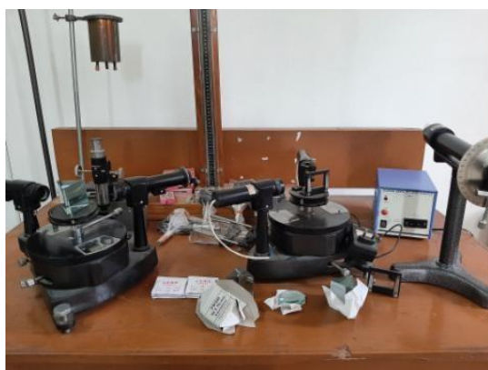
Optics experiment setup for interference, spectroscopy experiments using Laser and Sodium vapour lamp source N.B. Taken out of dark room for display purpose only
